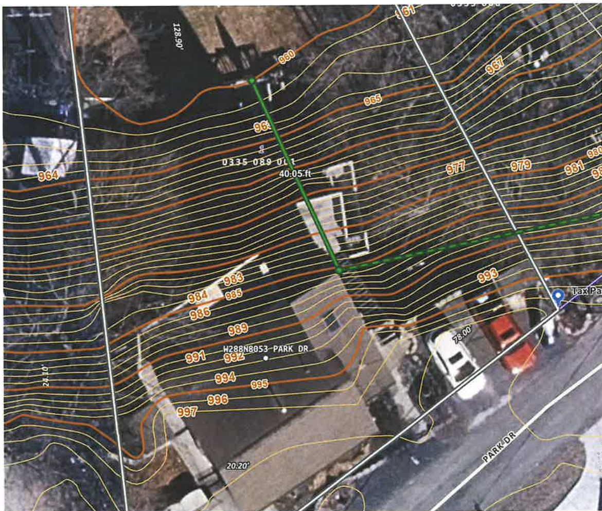
Figure 1 – Site Aerial Showing 1 Foot Contour Lines and Distance Measurement from Lawn Area to Northeast Corner of Residence (approximately 40 feet)
