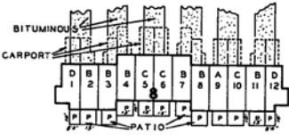
TYPICAL BUILDING SHOWING UNIT NUMBERS, STYLES, PATIOS, CARPORTS AND BITUMINOUS PAVEMENT.
