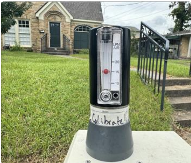
Air sample calibration set to 15 L/minutes
