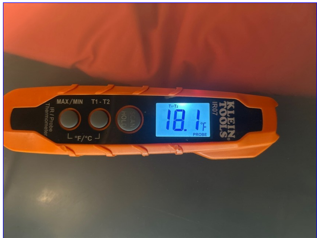
B. Item 3 (Picture) View of the measured delta T across the indoor component of cooling system 1
