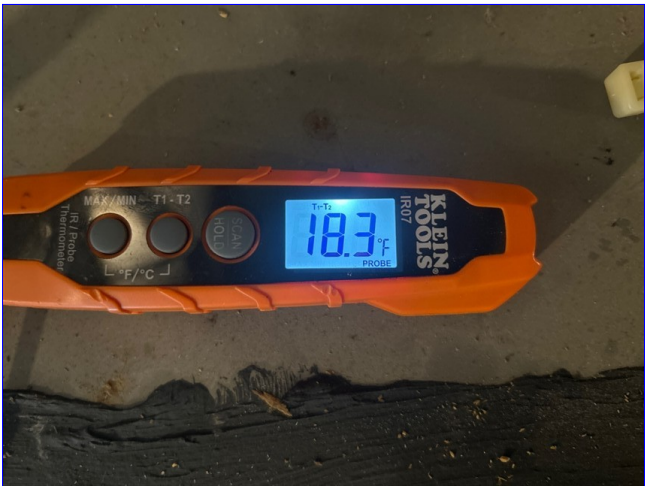
B. Item 2 (Picture) View of the measured delta T across the indoor component of cooling system 2
