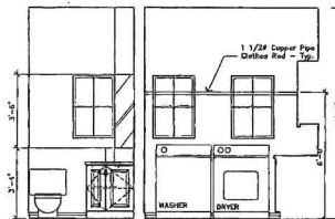
5 INTERIOR ELEVATION Toilet/Laundry 3/8 = 1-0
