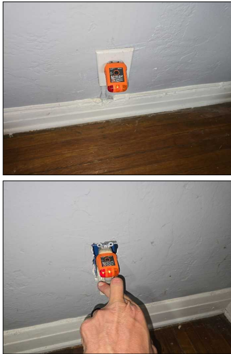
Outlet hot wired in reverse with neutral - needs to be serviced
