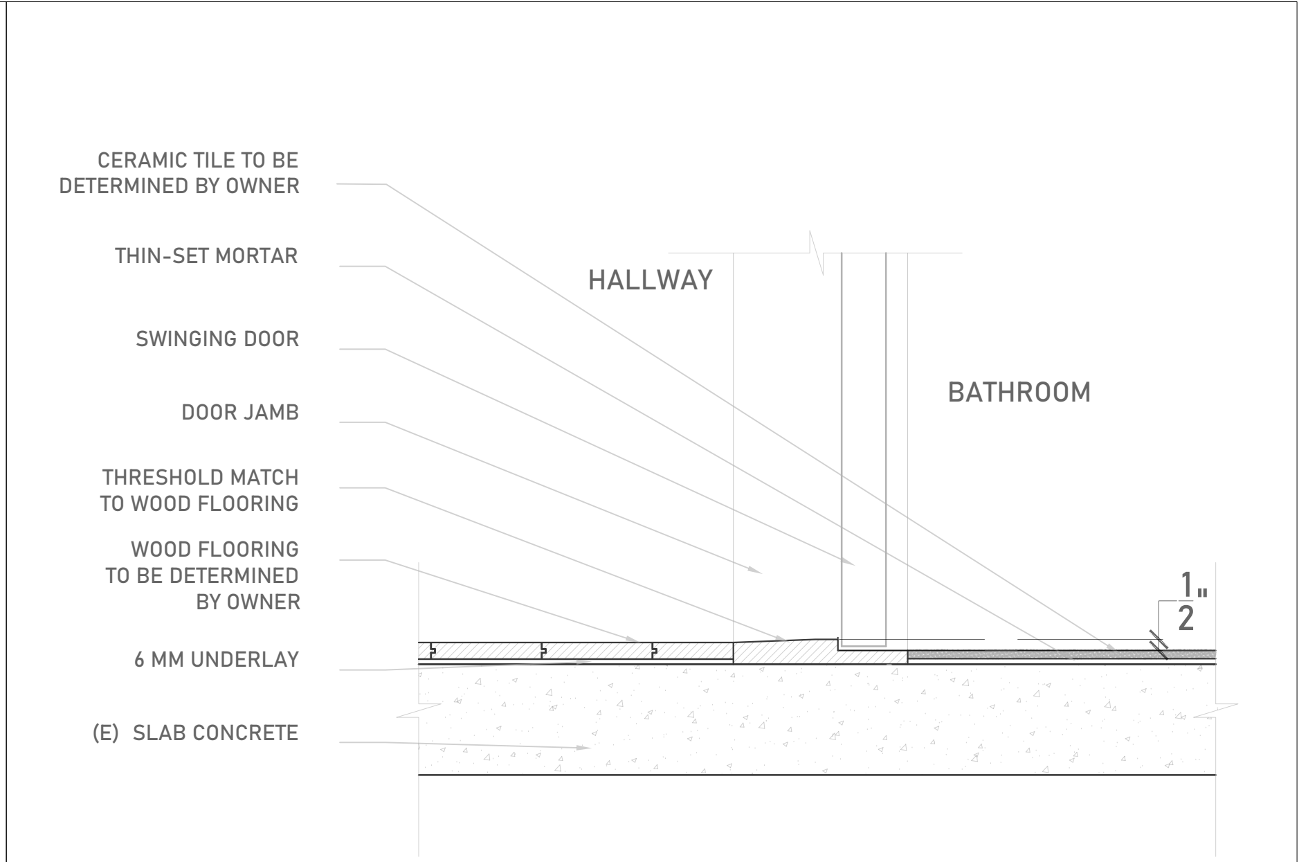
2 INTERIOR DOOR TRESHOLD ESC. 2" = 1'-0"
