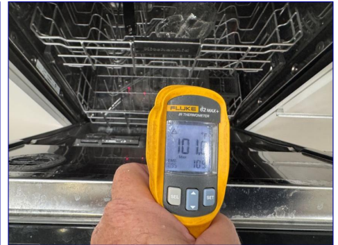
The dishwasher was turned on and tested by running for a short wash cycle and tested with an infrared thermometer, which shows the heated water inside the dishwasher. The photo serves to show the dishwasher was found to be functional when tested at the time of the inspection.
