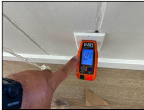
Three prong outlet(s) not grounded - needs to be serviced
