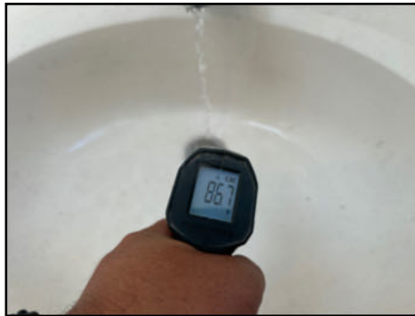
Hot valve did not function properly - needs to be serviced
