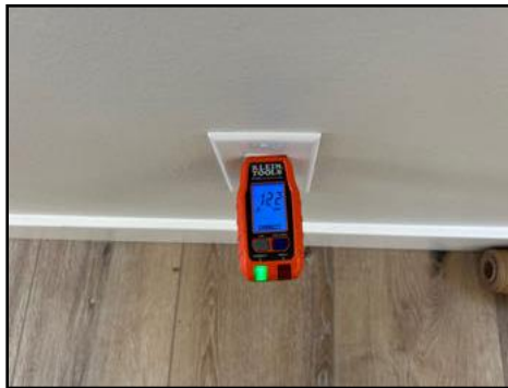
Three prong outlet(s) not grounded - needs to be serviced
