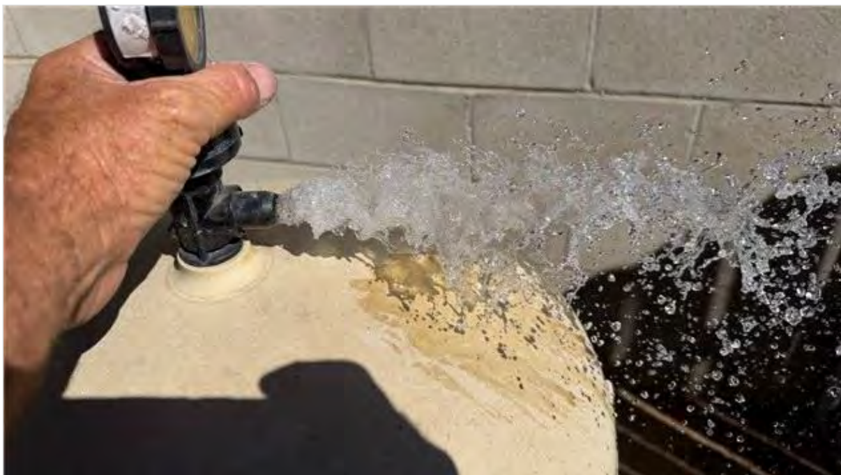
Filer Pressure Test
