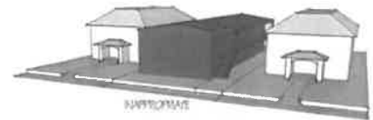
The infill example shown ignores the setback and entrance orientation of its neighbors
