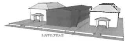
The in-fill example shown ignores the setback and entrance orientation of its neighbors
