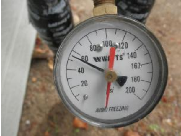
The water pressure was measured at 55 psi.
