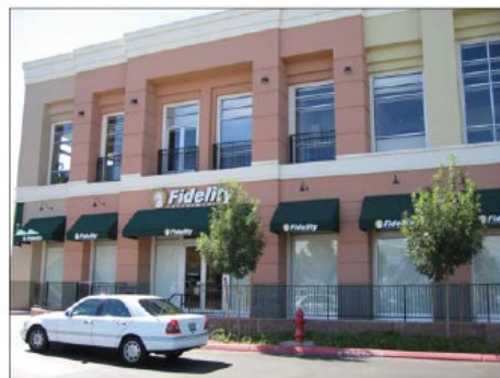
Smaller building bays can be articulated by color and material changes, as well as variations in the wall plane.
