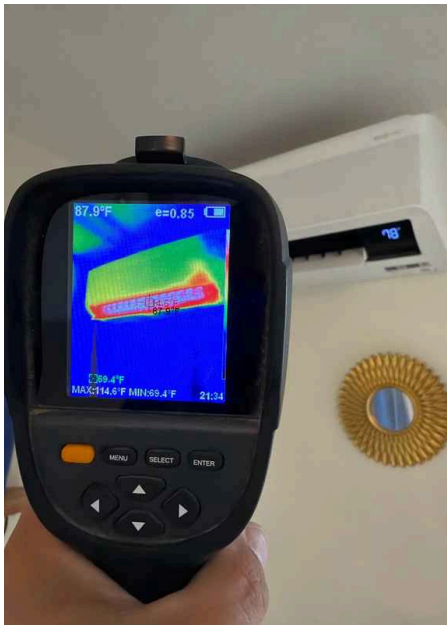
Cooling function on all heat pumps operational at time of inspection.
