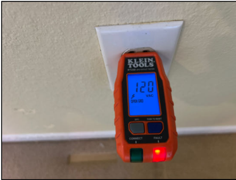
Three prong outlet(s) not grounded - needs to be serviced - multiple locations
